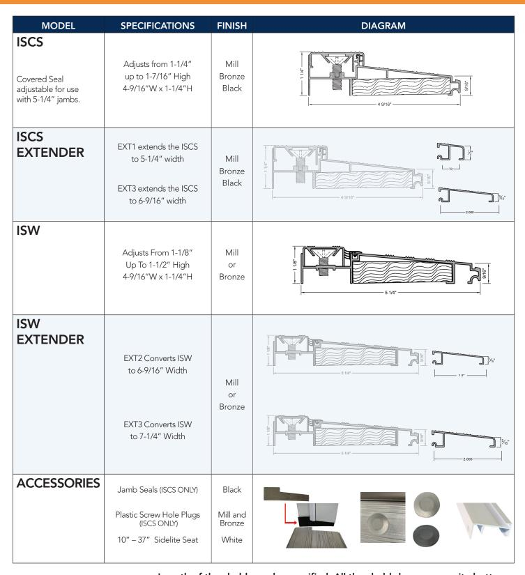
Length of thresholds can be specified. All thresholds have composite bottoms.
