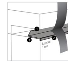
1. Top fin compresses as door closes, creating a seal between the header and the top of the door. The fin creates a barrier that directs water over the edge and down the exterior of the door.
